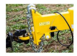
PIN MUST ALWAYS BE FULLY INSERTED INTO BREAKAWAY SWITCH. REMOVING PIN (AS SHOWN) WILL ACTIVATE BRAKES, & MAY DAMAGE TIRES, BRAKES, BATTERY, WIRING, & OTHER PARTS.
